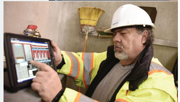
VTSCADA screens now allow remote monitoring of pump station status through the KISM web portal.
