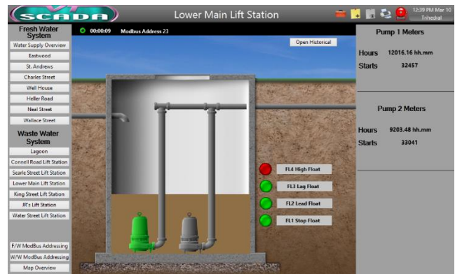
A custom SCADA display created using drag-and-drop tools.
