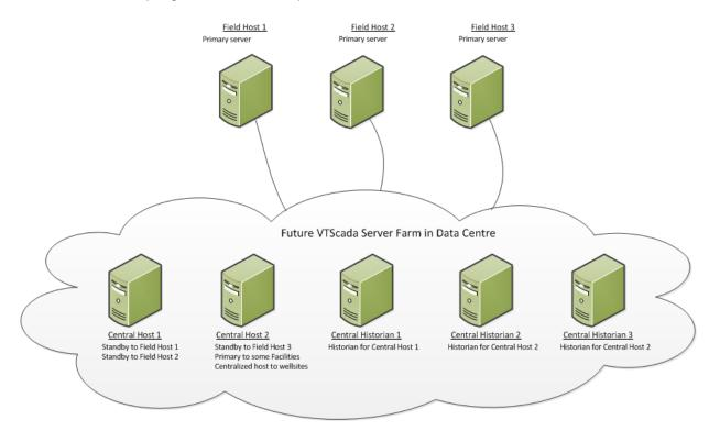
Having all of the data replicate to a central server farm allows a single interface to other corporate systems such as field data capture, measurement and data visualization systems. This model simplifies configuring a connection to each of the 200 existing SCADA hosts in the field today. The initial system design criteria contemplated 7 Million I/O without rationalization.
